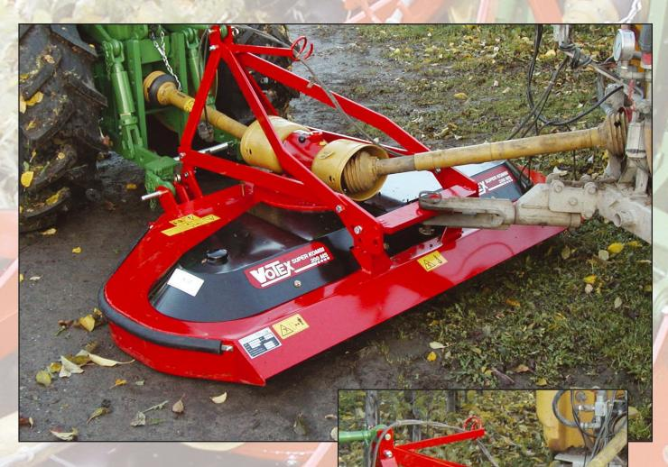
With the Super Kombi, Votex has developed a rotary mower which, when provided with a mowing-spraying frame, makes it possible to mow and spray in one operation. The Super Kombi is a compact rotary mower featuring a low construction, a very strong frame and three triangularly arranged cutting rotors resting on vertically adjustable supporting dishes. This construction guarantees excellent adaptation to the ground and a very stable movement even at high speeds.
