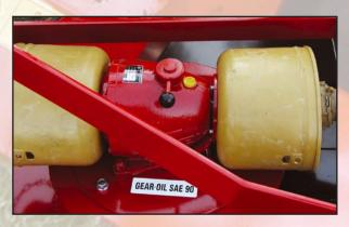
The machine is particularly suitable to be used in combination with an orchard sprayer. The disengageable gearbox enables spraying without mowing. It can also be used to stop the mower when filling the sprayer.
