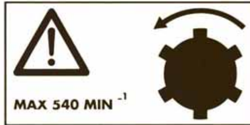
Picture 5.1 RPM and direction of rotation PTO
