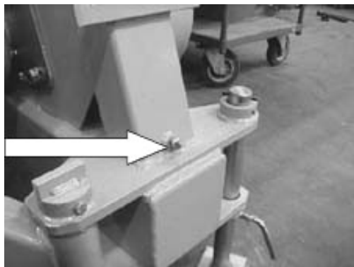
Picture 9.4.1 Draining leaked oil
