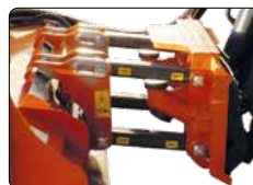
Attacco SAE J2513. Universal coupling SAE J2513.
