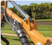
Arms with circular section H.T.R. (High Torsion Resistance).
