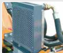
Oil cooler with thermostat (option).
