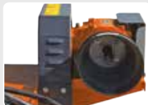
Gearbox external to the gear housing.
