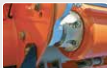
Rear roller support with internally fixed bearings NG without grease fittings.
