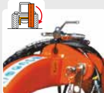
Flailhead hydraulic lock tap for transport (no chains or brackets).
