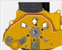
Inner lining "Full coverage" Domex 700 Steel.
