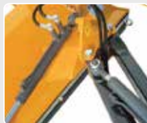
Rotation joint and arms mounted on self-lubricating bushes.
