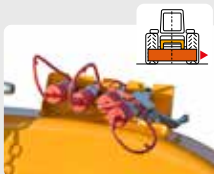
Hydraulic lock tap for transport. Manual engagement (no chains, no brackets).
