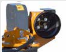
Gearbox external to the drive housing.
