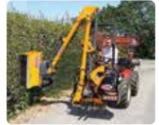
Version 320A/R For front mounting on tractors with reversible drive.
