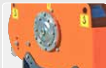
Rotor support with bearings positioned inside the frame.
