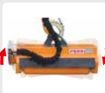
Floating head system to follow ground contours.
