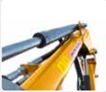
Arm with circular section H.T.R. (High Torsion Resistance).
