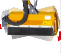
Floating head system to follow ground contours.
