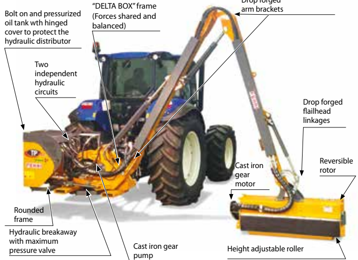
Floating head system to follow ground contours.
